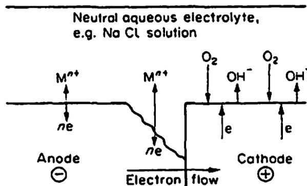
Figure 1: Basic Corrosion Cell
